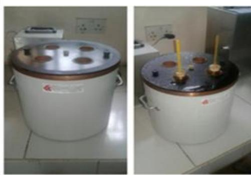
Figure 5: Cloud and pour point chamber with test jar inserted
