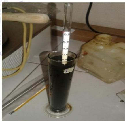
Figure 2: Specific gravity of a crude sample being determined with a hydrometer
