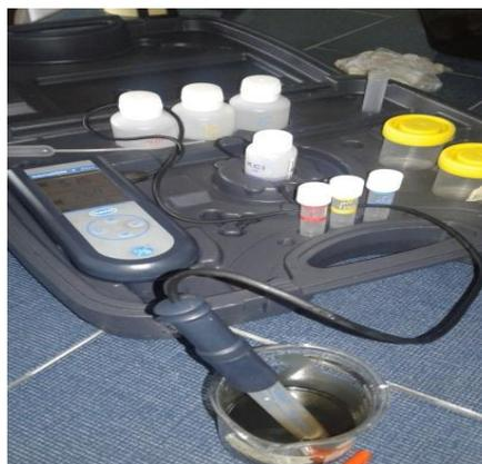
Figure 1: Hanna pH meter determining the pH of a crude sample
