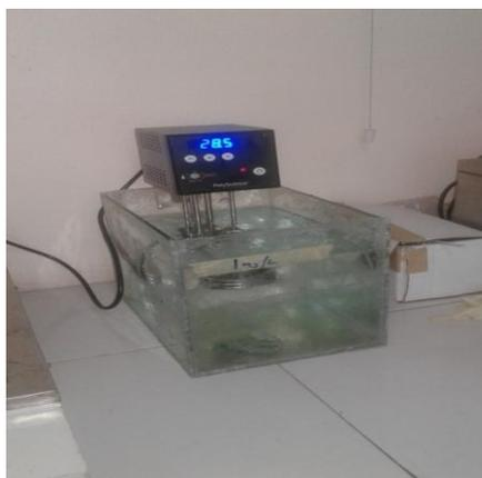
Figure 3: Water bath and heater
