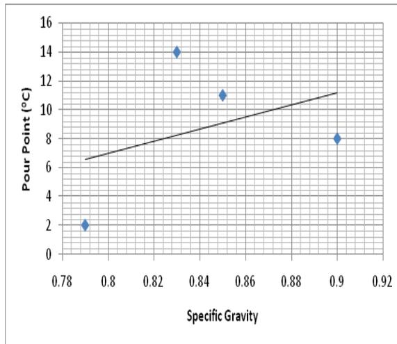
Figure 7: Graph showing relationship between specific gravity and pour Point.
