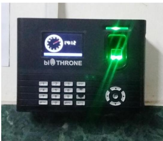
Fig.1: Biometric Fingerprint Capture Device
