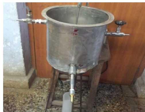
Fig 1: Activated Sludge Tank
