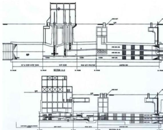
Figure 4: Gates Arrangement at North Junction Box and South Junction Box
