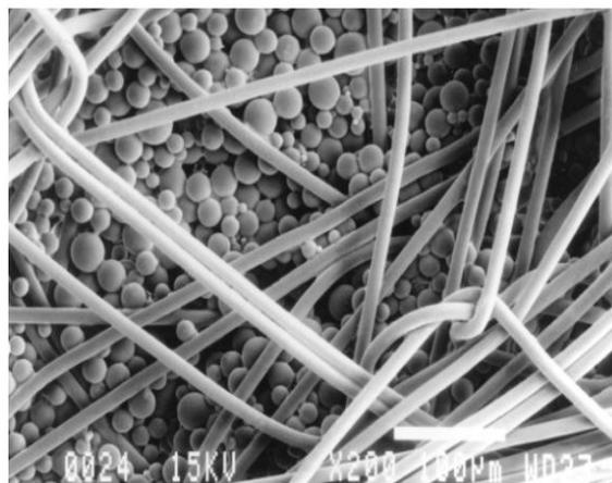
Fig. 4 PCM microcapsules in a fabric (Outlast Europe).
