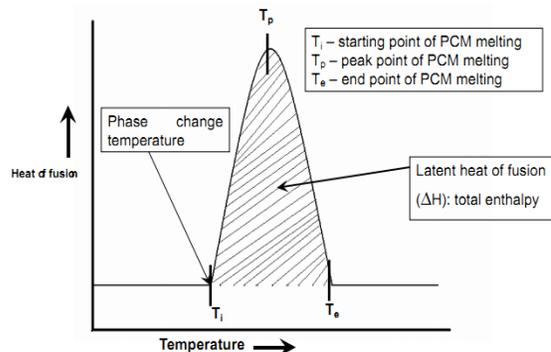
Fig. 3. Schematic of DSC heating thermogram of PCM. [21]
