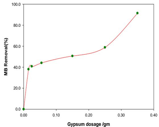
**Fig.4.** Effect of adsorbent dosage on the adsorption of MB on gypsum, [MB] =  $2.0 \times 10^{-5}$  M, pH 6.0, contact time 60 min, at room temperature.
