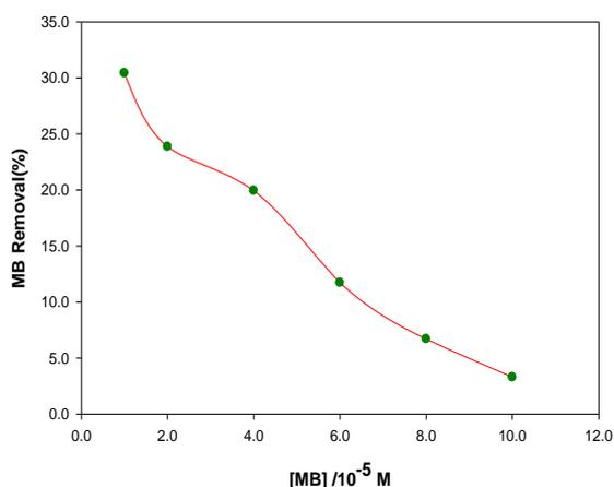
Fig.6. Change in adsorption of Methylene Blue on gypsum with its concentration, amount of gypsum = 0.025 g, contact time = 60 min, pH 6.0, temperature =25°C.
