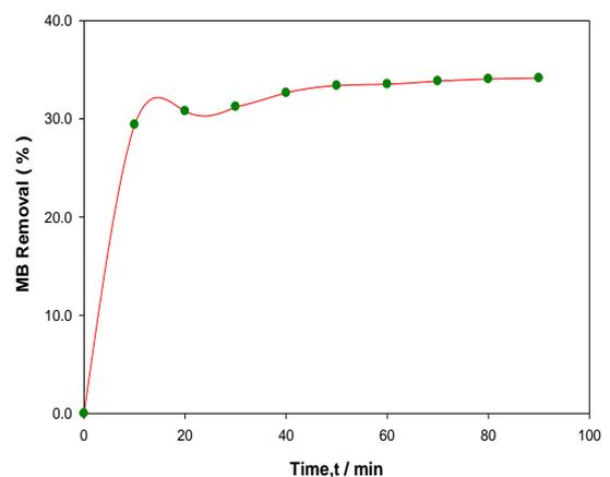
**Fig.5.** Change in adsorption of MB on Gypsum with time, [MB] =  $2.0 \times 10^{-5}$  M, Gypsum = 0.025 gm, pH 6.0, contact time 90 min, temperature =  $25^{\circ}C$ .
