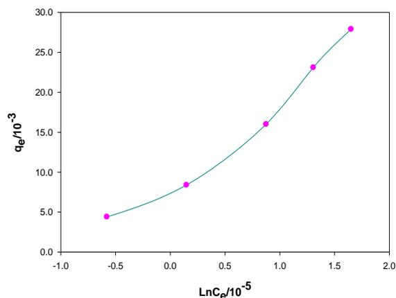
**Fig. 9:** Tempkin isotherm of MB adsorption On Gypsum, Gypsum= 0.025 gm, [MB] =  $2.0 \times 10^{-5}$  M, contact time 60 min, pH 6.0,
