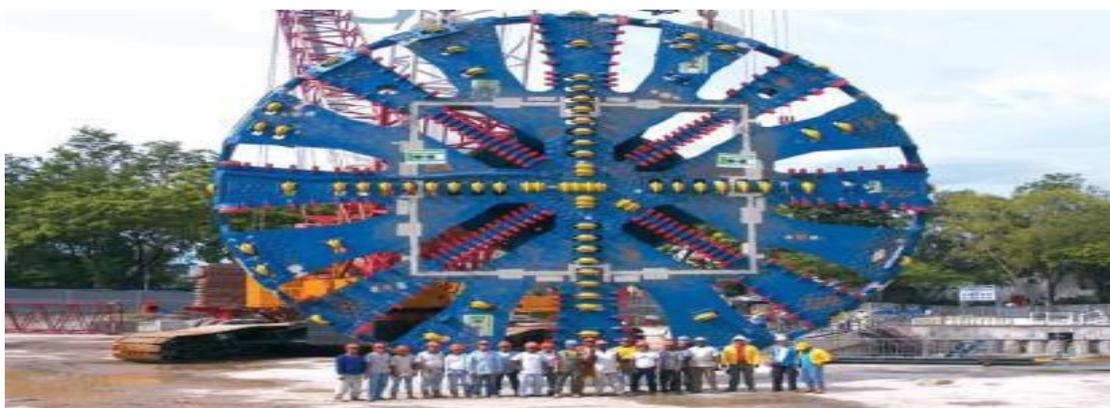
**Figure 4: The Slurry Shield TBM at SMART Project**
