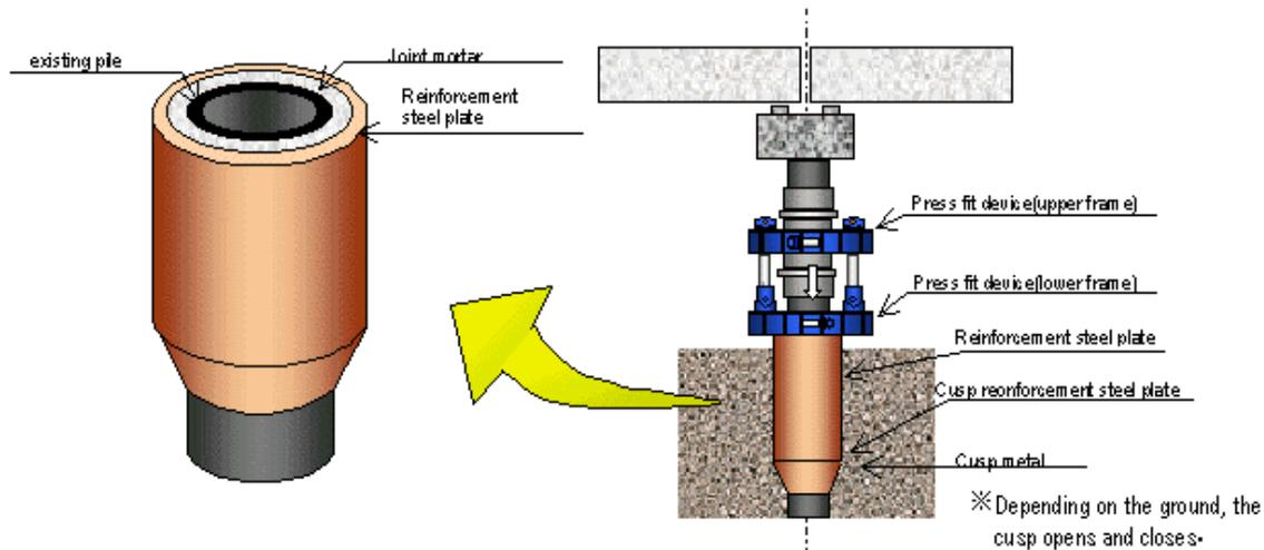
**Figure 8: Method Protect the piles**
